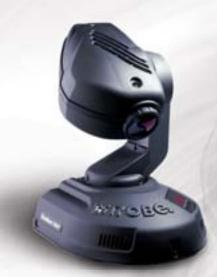
The ClubSpot 150 CT has the similar ultra compact effect luminaire as ClubSpot 160 CT, which includes colour wheel with 11 dichroic filters and static gobo wheel with 11 metal gobos; variable strobo effect; shutter and manual focus. The ClubSpot 150 CT achieves a high level of performance for clubs & bars and discotheques applications.
