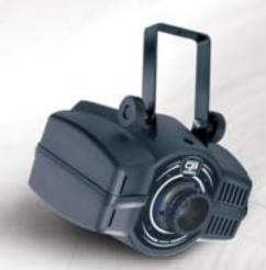
The FLARE is fully DMX controlable spotlight projector. It comes to the market with 19° beam angle, colour wheel with 15 dichroic filters, powerful 250W halogen lamp, a strobe effect and additional control option of "auto-trigger" or "music-trigger".
