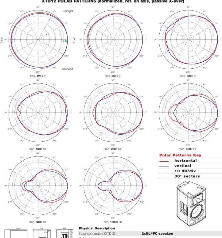
Cabinet: material birch plywood curved deflector with convex-concave shape additional device HDSC™ XT-KITDEF (3 flying tracks) Suspension system Dimensions (WxHxD) 410x635x432 mm Net weight (XTD12) 31.5 kg Net weight (XTD12/A) 33 kg
